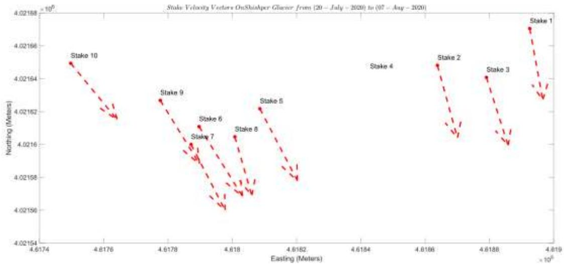
Figure 4: Velocity vectors of the stakes (Stake No. 1 to 10) at the snout of the Shishper Glacier are presented. Easting and Northing are presented with distance in meters from central meridian i.e., 75°E and from equator, respectively. The stakes have moved 7.4 meters from July 20<sup>th</sup>, 2020 to August 7<sup>th</sup>, 2020 ( 17 days) at the rate of ~43.6 cm/day in southward direction and 1.7 meters east ward at the rate of 10 cm /day.
