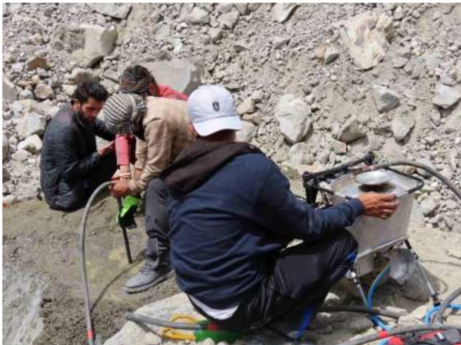
Figure 3: a) Stake 15 installed for assessment of surge in Shishper Glacier on July 21st, 2020. b) Hole on Shishper Glacier is being drilled using Thermal Ice Drill.
