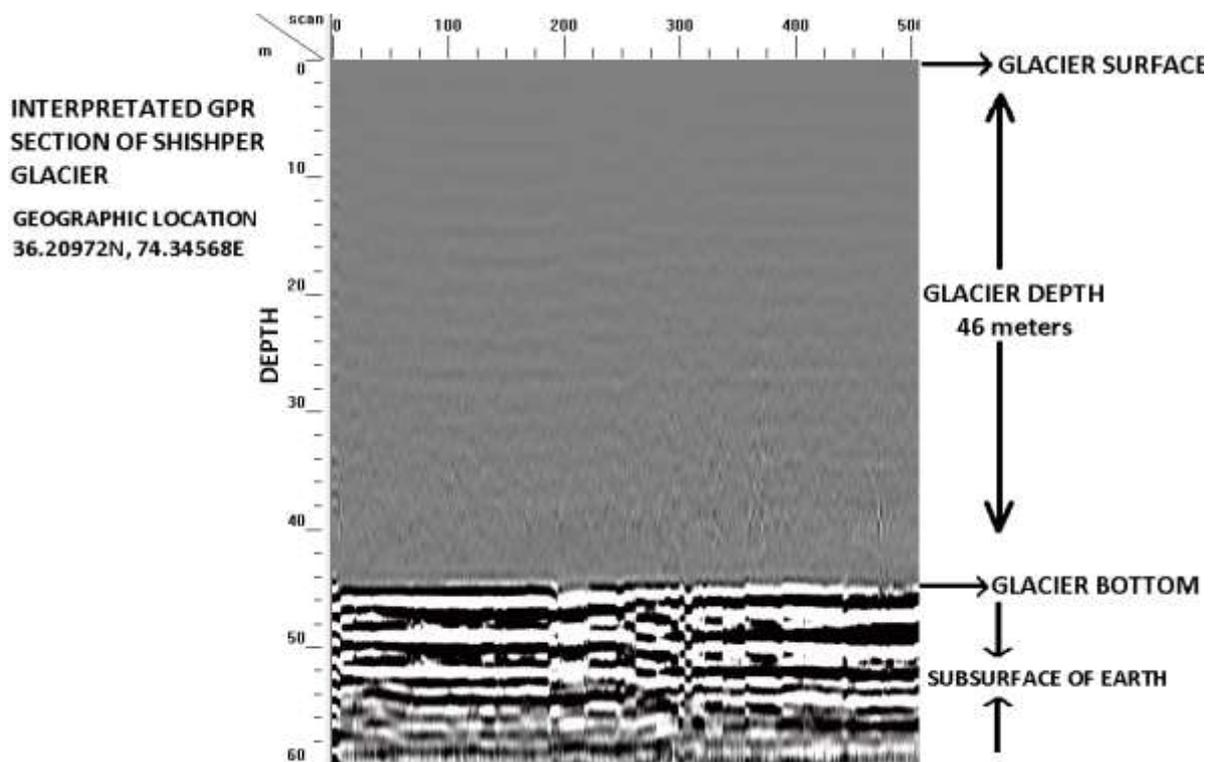
Figure 6: Depth of Shishper glacier was estimated on several locations near snout using Ground Penetrating Radar (GPR). It was around 46 meters deep. Regular monitoring of Shishper Glacier depth through GPR will help to assess its future behavior. In case of retreat, the depth is start decrease, whereas in case of surge it either will accumulate more mass, or may sustain same depth.
